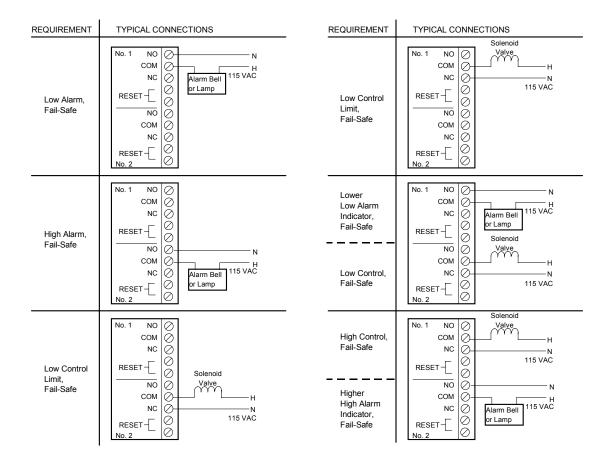
Figure 2-6. Relay Terminal Connections for Typical Fail-Safe Application
